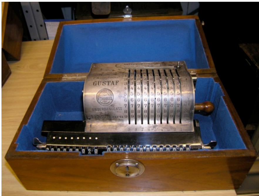
Figure 20. Odhner arithmometer nr. 852 (capacity 13) at the National Museum of Science and Technology, Stockholm. This calculator was produced in January 1892 and is the gift of the inventor to Crown Prince Gustaf.
