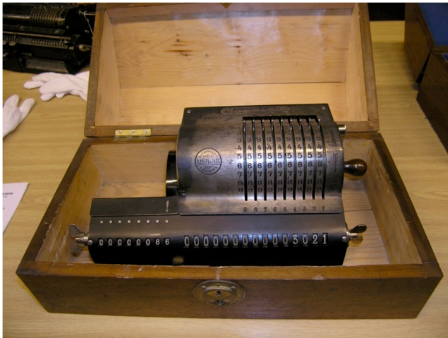
Figure 23. Odhner–Hill arithmometer nr. 1148 of the National Museum of Science and Technology, Stockholm in an original case. This is the first known 15–digit model. The coverplate here is nickel–plated, which was at that time cheaper than a lacquered coverplate [96], see also Figure 26.
