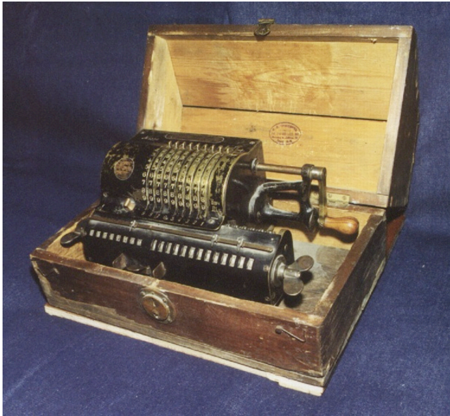
Figure 24. Odhner–Hill arithmometer nr. 1326 of Sergei Frolov, photo ©Sergei Frolov. The case is original, but the long crank, decimal pointers and input lever clearing system have evidently been refurbished later. The number wheels here (as in arithmometer nr. 1209) have black numbers on a white background.
