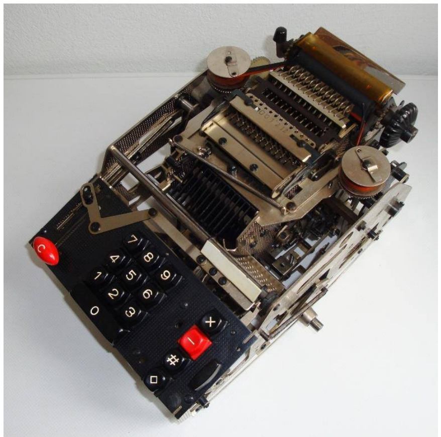
Fig. 4: Romanoni Model Wunder , S/N 001.612, without casing.
