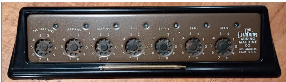
Fig.: The result of 10 \div 7 on a Lightning Adding Machine (1.4285 + 5 as remainder)
