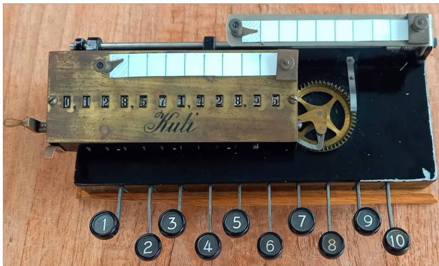
Fig.: The result of 90 \div 7 with 10 significant digits and a remainder on the Kuli, a simple column adder with a tens transfer in three columns.
